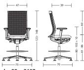
due88 + 3107 with arm supports: 21 kg without arm supports: 19 kg
