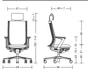
due99 / due98 with arm supports: 20 kg / 19 kg without arm supports: 18 kg / 17 kg
