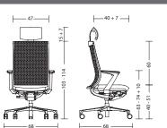
due89 / due88 with arm supports: 20 kg / 19 kg without arm supports: 18 kg / 17 kg
